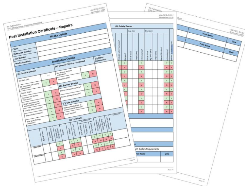
Figure 4.12 - Example of a VRS Installation Certificate
