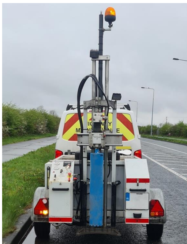
Figure B.1 - Trailer Mounted Coring Rig and Towing Vehicle
