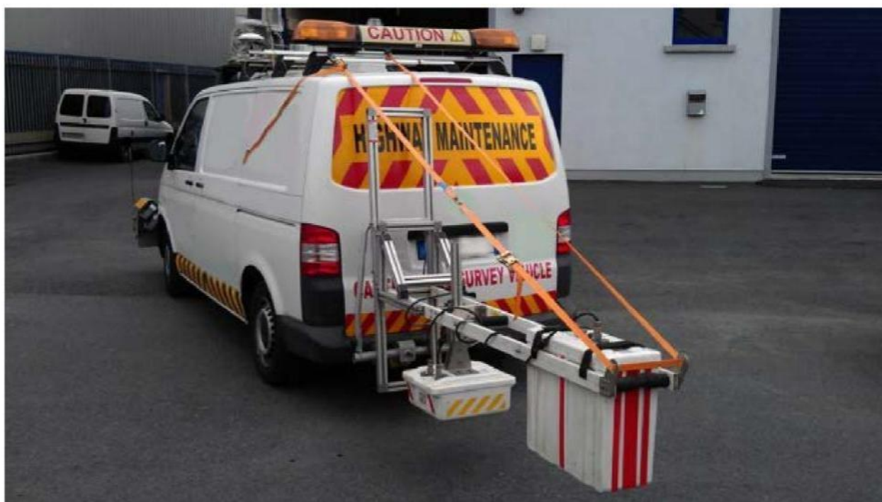
Figure A.1 - Typical Ground Penetrating Radar (GPR) Equipment
