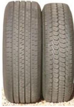
Figure 3.3 - CPX-tyres according to ISO/TS 11819-3: P1 (left: Uniroyal Tigerpaw 225/60 R16) & H1 (right: Avon Supervan AV4 195R14C)
