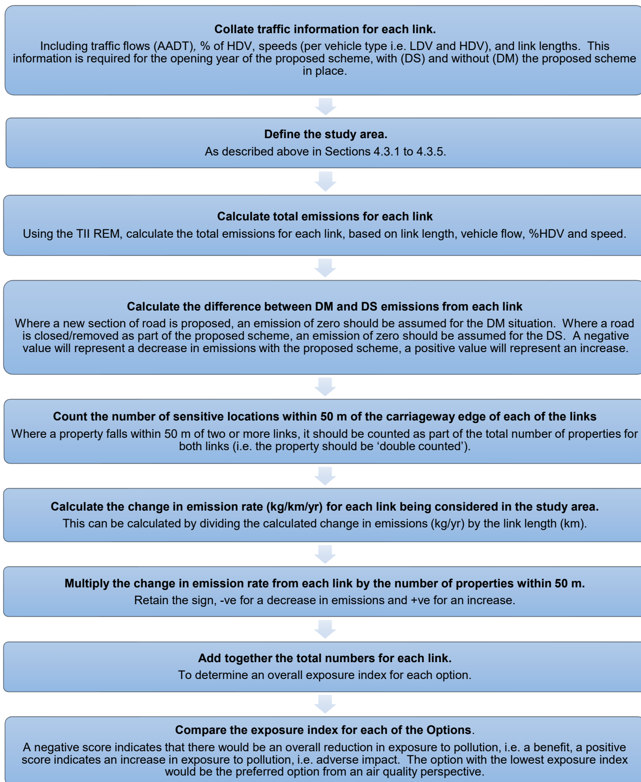
Figure 4.4 Summary of steps to calculate the Index of Overall Change in Exposure
